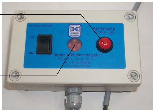
Fig 8b. Press and hold the activation button until Quick Hitch hooks have fully retracted.
